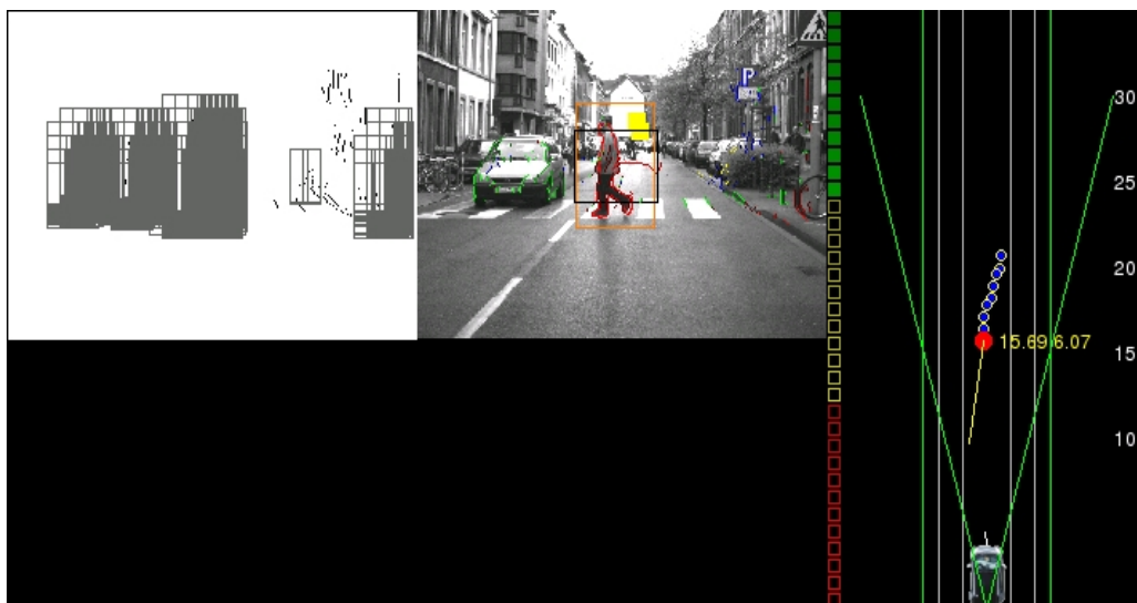
Figure 12: Output of SAVE-U Configuration B. Left window shows results of stereo-based object detection (grey bounding boxes). Middle window shows correctly recognized pedestrian (red shape). Right window shows a top view of situation in front of vehicle: pedestrian at current/previous time instances shown by red/blue dot. Right hand scale is given in meters.
