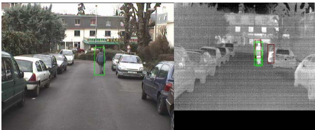
Figure 5: Same as Figure 4. In addition to the correctly recognized VRU, a false ROI from the detection module was correctly rejected by the classifier.
