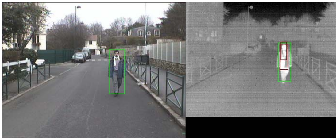
Figure 4: Example of a VRU correctly recognized by the vision system. The right sub-image shows the classification results superimposed on the FIR image. Green boxes denote ROIs classified as VRUs, ROIs rejected as non-VRUs are shown in red. The left sub-image displays the output of the tracking module superimposed on the color image.
