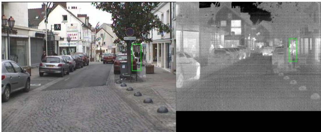
Figure 8: Another example of a false positive: Although the image ROI contains a VRU, the position of the box is incorrect.
