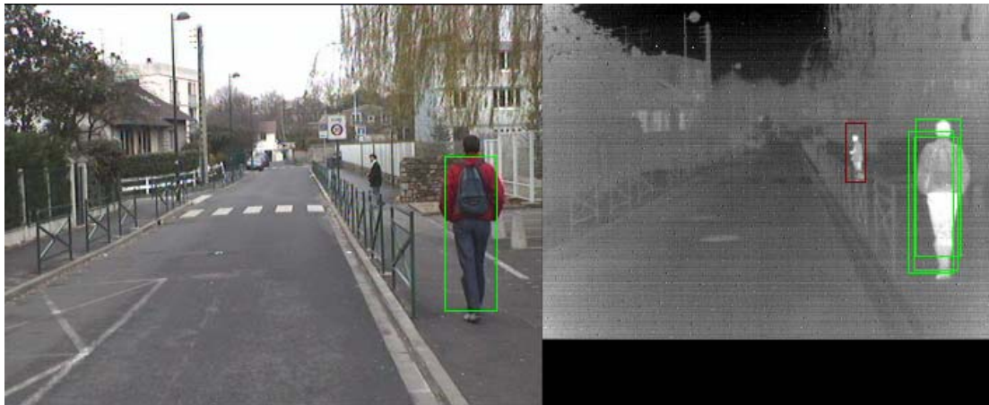
Figure 10: Another example of a missing recognition: The second more distant pedestrian was misclassified as a non-VRU.
