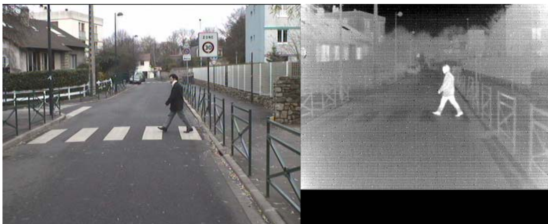
Figure 9: Example of a missing recognition: No ROI generated by the detection module.
