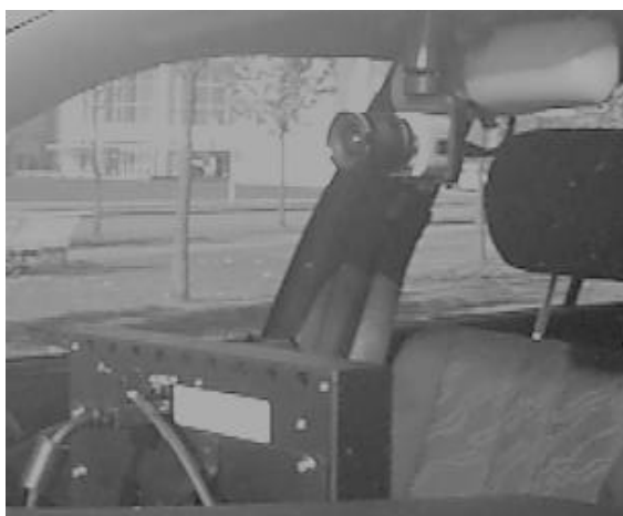
Figure 1: Video camera mounted on-board the DaimlerChrysler test vehicle.
